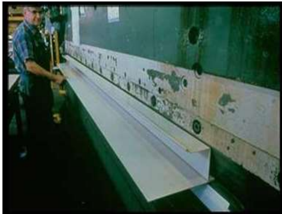
Figure 1: Example of Press Brake Operation
