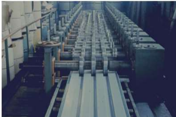
Figure 2: Images showing Rolled Formed Operation Un-stiffened Element
